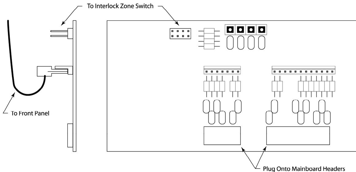
The shield board is now plugged onto the headers on the main circuit board where the connectors used to be. Besides the pins of the header, there is no other mechanical means to mount the Shield, so be careful. Replace the MCU board being sure that there is an insulating layer between the Shield board and the MCU board.
